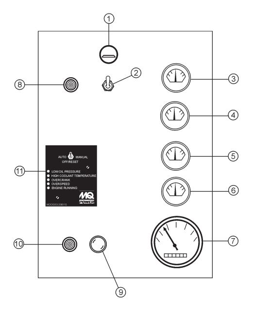
Figure 7. Engine Operating Panel
